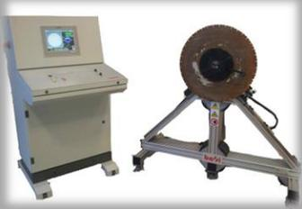
**Cten-PC** - Electronic tensioning control with PC for saw blades from Ø 230 up to 2000mm.
