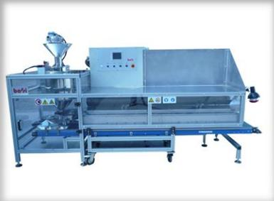
**Gran** - Designed to run automatic granulation processes of metal powders with or without diamond.
