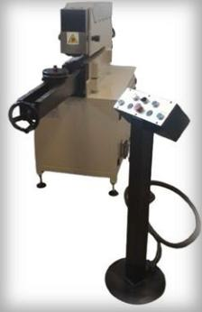
**Ten 1600H** - Hydraulic tensioning machine for saw blades from Ø 300 up to 1600mm.
