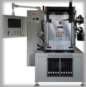
**Sint 150VDP** - Sintering machine with square Vacuum chamber equipped with Digital Power unit. Maximum Power 150 kW, maximum pressing force 80 Tons.
