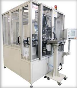
**GCP2** - Gravimetric Cold press with compression force of 26 or 42 Tons. The dosing machines are positioned to the left and to the right of the mould, the weight accuracy is 0.01 g. The machine has two independent powder transportation carriage.
