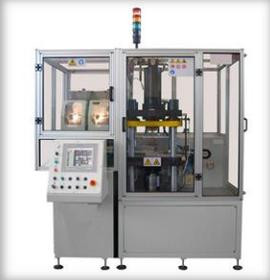
**GCP1** - Gravimetric cold press with compression force of 20 or 40 Tons. The dosing machines are positioned on the left side of the mould, the weight accuracy 0.01 g. The machine has a single powder transportation carriage.
