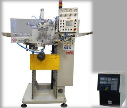
**Bra1 & 2** - Automatic brazing machine with 1 or 2 head for saw blades from Ø 230 up to 1600/2000mm.
