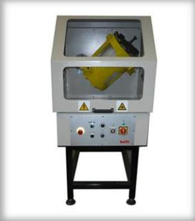
**Mixer** - Mixer for metal powders for 2, 5, 10 liters containers, produced to obtain perfectly homogeneous mixtures also in presence of elements with different specific weight.
