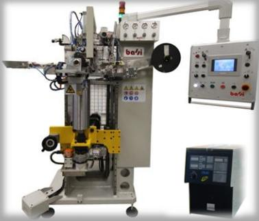
Bra1-CD - Automatic brazing machine for core drills from  $\varnothing$  80 up to 500/800mm.
