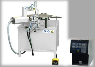
**BRM 2000** - Manual brazing machine for saw blades from Ø 230mm up to 2000mm and linear gang saws. The machine can be sold with or without HF generator.
