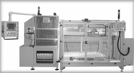
**Sint 150VDP + CSR Sint 30** - Sintering machine with round Vacuum chamber equipped with Loading/Unloading unit up to 30 frames complete of cooling station. Machine equipped with Digital Power unit. Maximum Power 150 kW, maximum pressing force 80 Tons.
