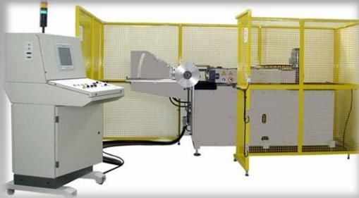
**Ten1600-PC / Ten2200 PC** – Full automatic tensioning machine for saw blades from Ø 300 up to 1600mm or up to 2200mm.
